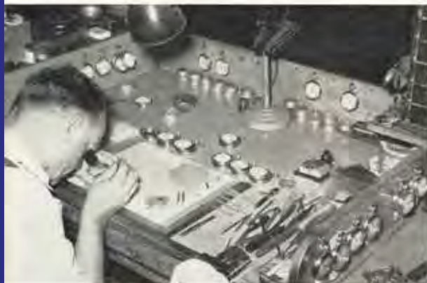
Above: Arthur Taylor delicately replaces the balance staff of a watch. Below: Reg Wrigley's machine cleans a watch in seven minutes.
