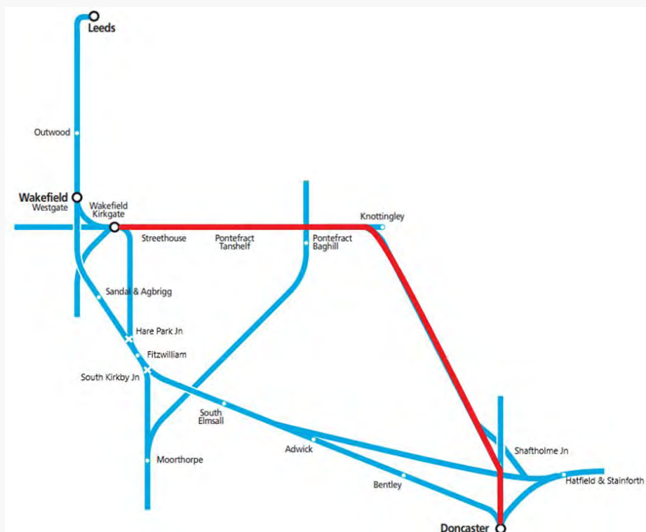
Figure 24: Simplified diagram showing the re-routing opportunity via Shaftholme Junction and Knottingley
