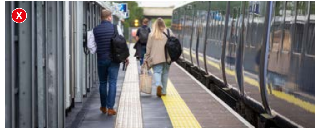
Image 2.5.5.1: Do not install a tactile guidance path on a narrow section of the platform without maintaining the minimum exclusion safety zone of 1200mm from the tactile platform edge warning
