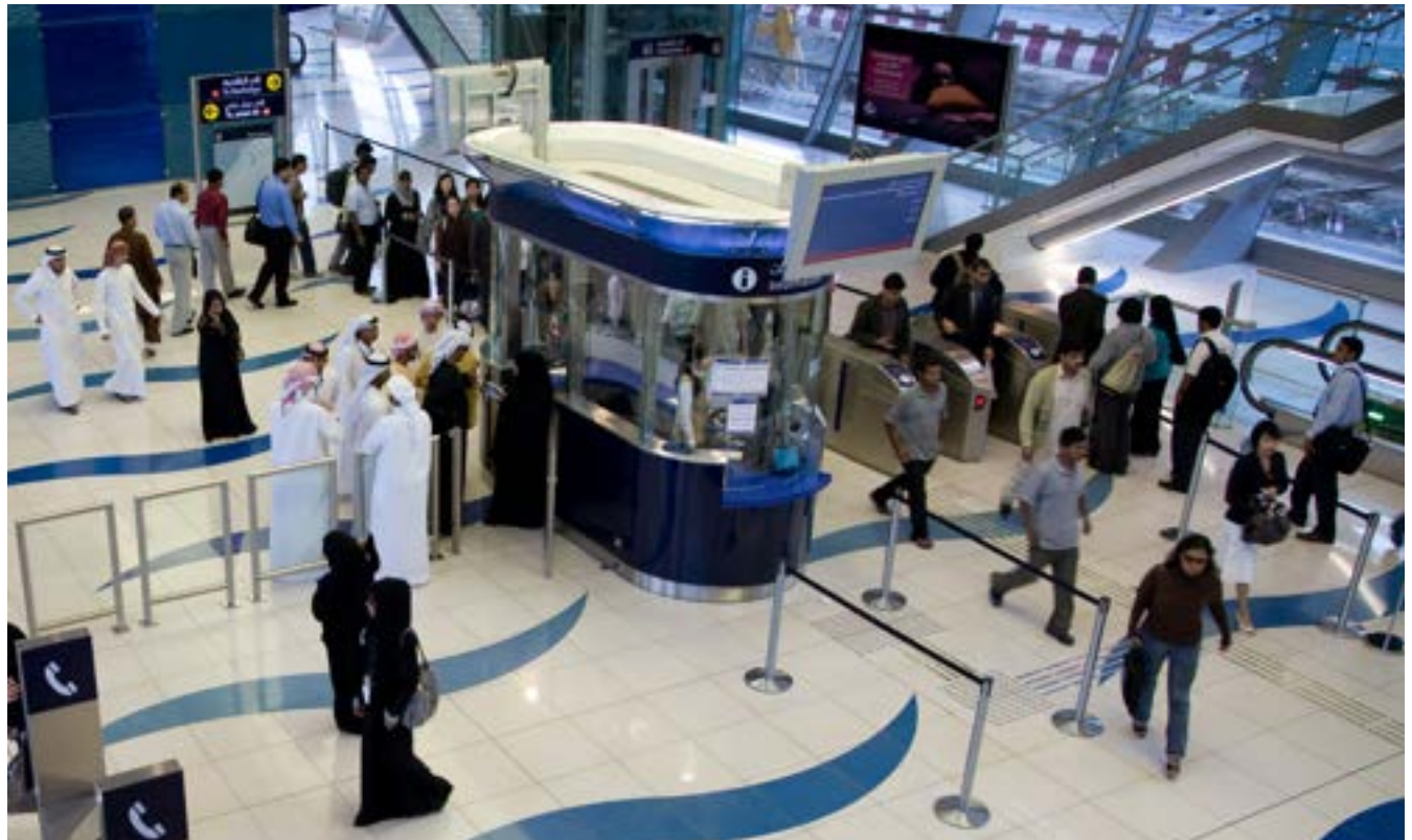
Image 1.6.1: Example of a Tensor barrier obstructing a tactile guidance route in a Dubai Metro Station
