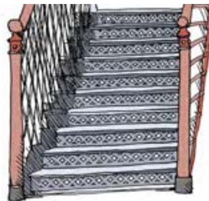
Image 6.3 Existing, Non-compliant Features. Example of open risers that are not permitted on electrified lines.
