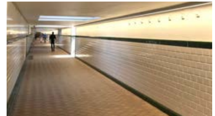
Image 8.3 In this narrow and low tunnel the linear luminaire is asymmetrically positioned to highlight one of the walls. The bluish skylights are artificial.
