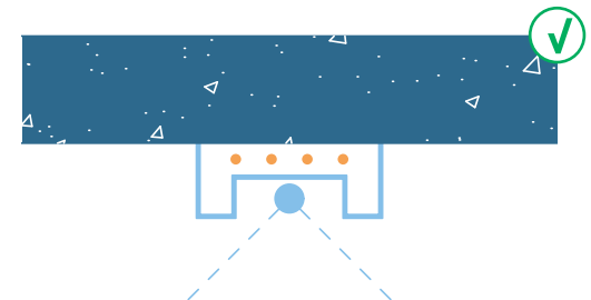
Image 9.13 Luminaire with integrated cable management to avoid secondary CMS.
