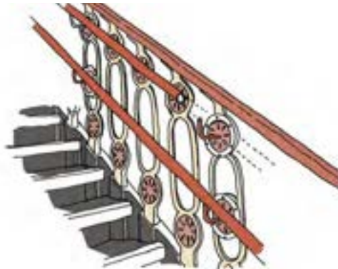
Image 6.2 Upgrading Handrails. Example from Llanfairpwll station footbridge.
