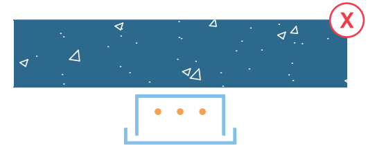
Image 9.12 Surface mounted conduit with lid, typically galvanised steel. Widely used but should be avoided in preference of more integrated solutions
