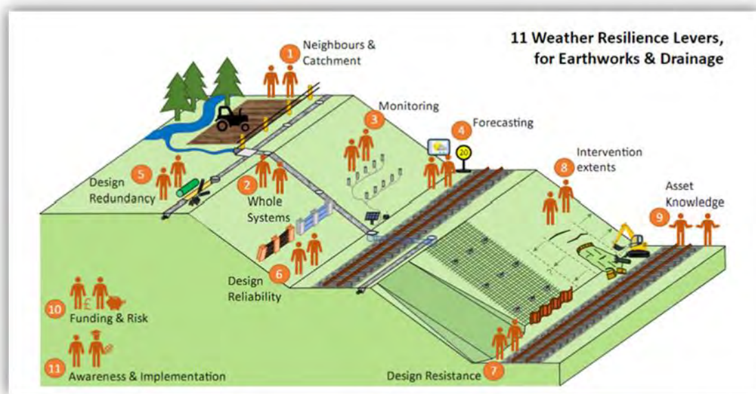
Figure 5.3-1: 11 Weather Resilience Levers for Earthworks & Drainage.
