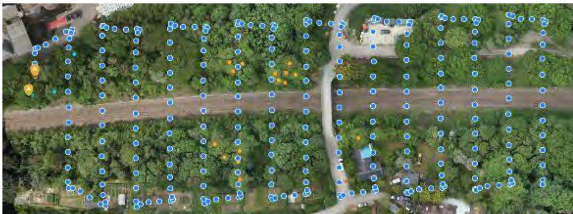
Figure 7.1: Drone data, with blue points representing individual photographs stitched together to create the map and model, which subsequently reveal the flight path taken by the drone. Other points identify individual trees either for their health or size.
