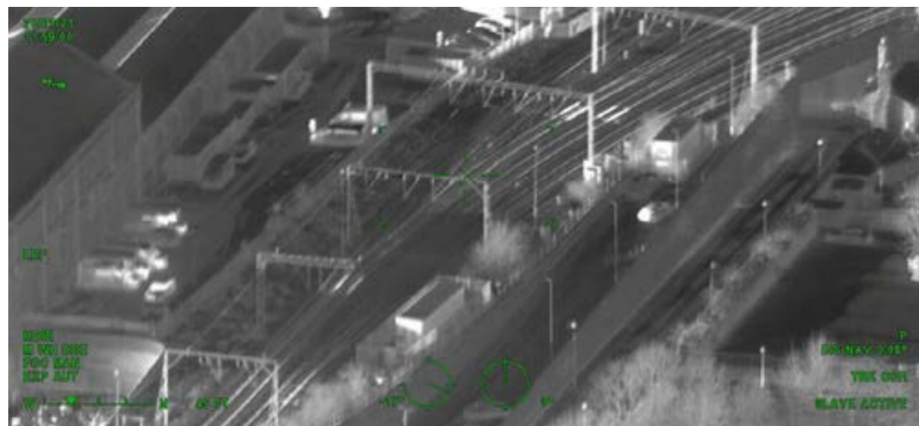
Figure 32) Aerial thermal image showing heated points on approach to Wolverhampton station. Source: Aerial thermal image showing heated points on approach to Wolverhampton station – Network Rail Air Operations team (networkrailmediacentre.co.uk) (networkrailmediacentre.co.uk) Credit: Network Rail Air Operations Team.
