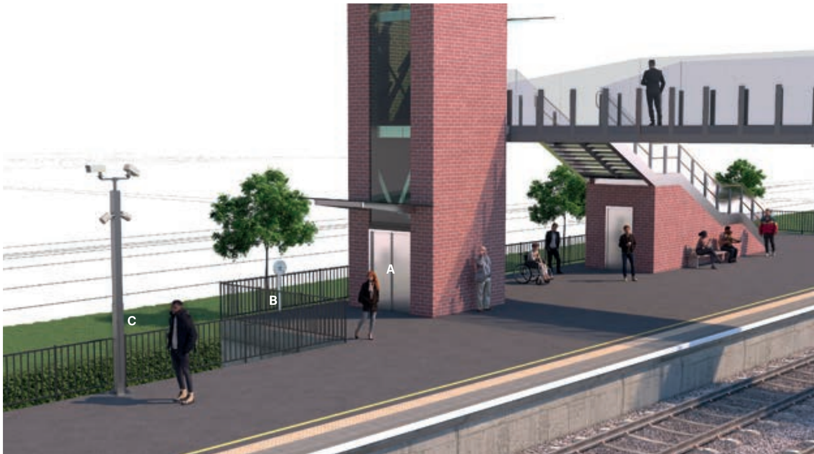
Figure 17 Indicative image showing the provision of EVC, CCTV and Public Address to support beneficial use of passenger lifts for evacuation
