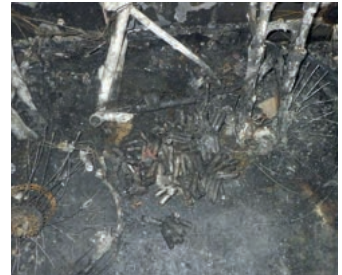
Image 10.5 Aftermath of an e-bike fire caused by a lithium-ion battery ©London Fire Brigade
