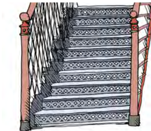
Image 2.3 Existing, Non-compliant Features Example of open risers that are not permitted on electrified lines.
