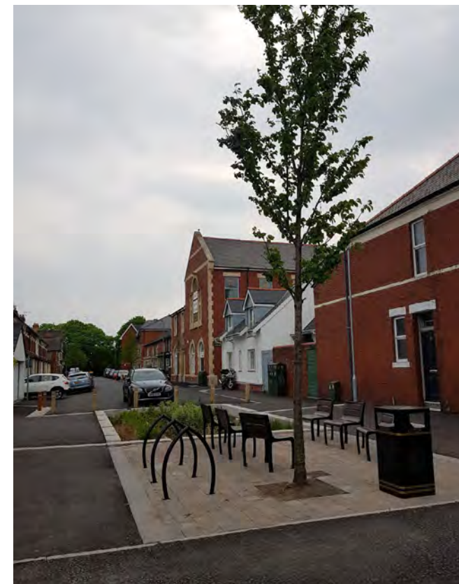
Figure 47. Permeable paving used for the Grangetown Project in Cardiff. Source: © Arup
