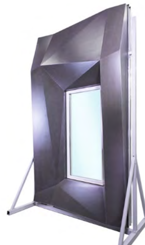
Figure 41. High Performance, Economical and Sustainable Biocomposite Building Materials, a €7.5m research project, explored the potential for biocomposites to reduce capital carbon in façades. For more information see https://cordis.europa.eu/project/id/285689/reporting . Source: Lichtzelt
