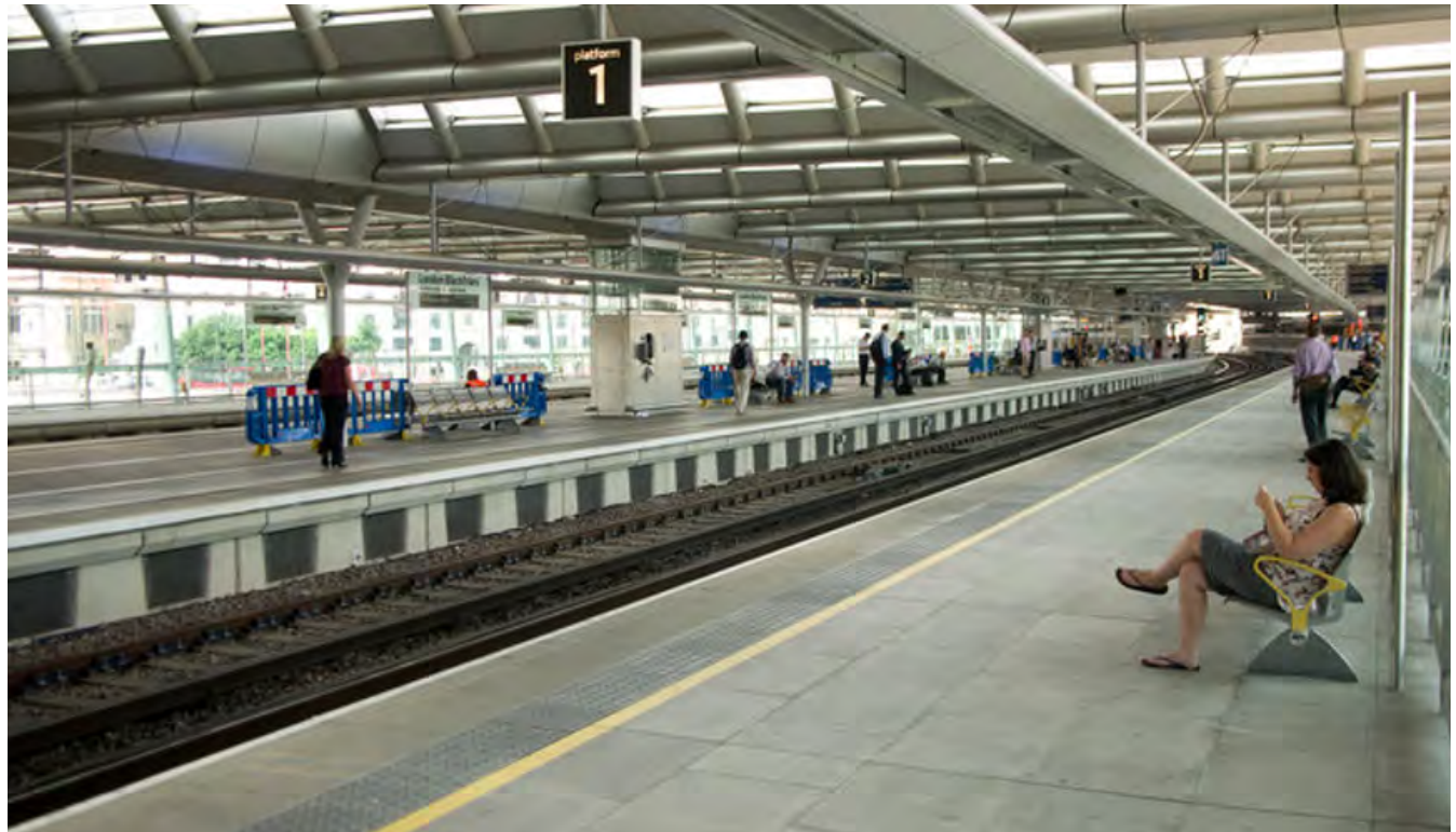
Figure 21. Platform-edge artificial lighting switched off on a bright day at Blackfriars Station thanks to north-lit platforms, without losing opportunity to generate renewable energy from south-facing solar PVs. Credit cc-by-sa/2.0 - © Julian Osley - geograph.org.uk/p/3570690
