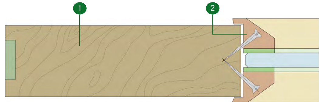
Figure 7.28: Indicative Sketch - Cross sections of door to vision panel
