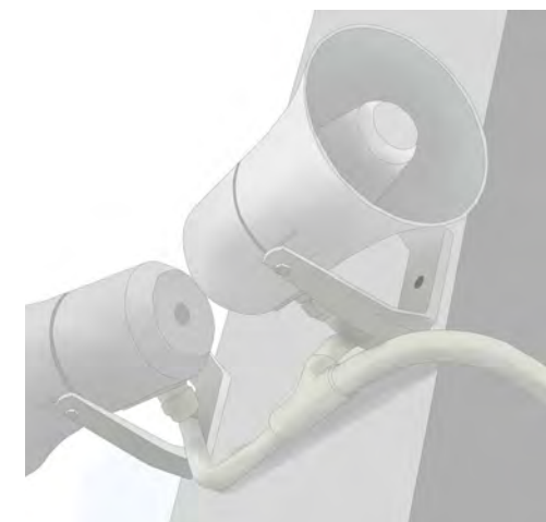
Image 12.12: Illustration of a PAVA loud speaker
