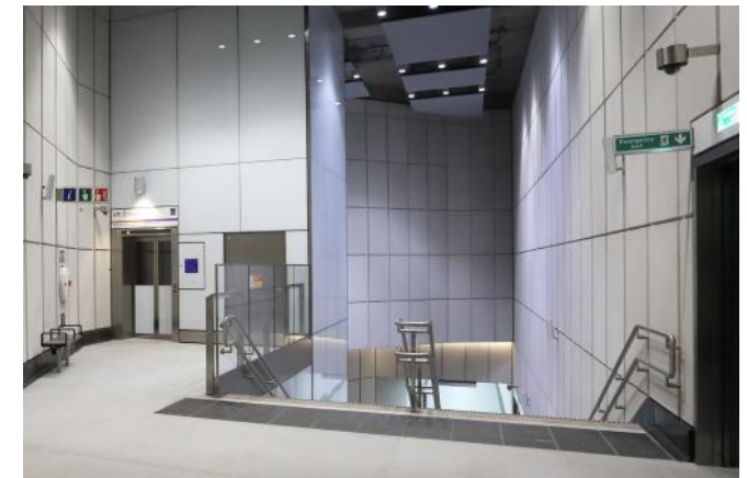
Image 2.4 At Liverpool Street Elizabeth line station, a new lift has been positioned in order to maximise visibility from both the upper and lower landings.
