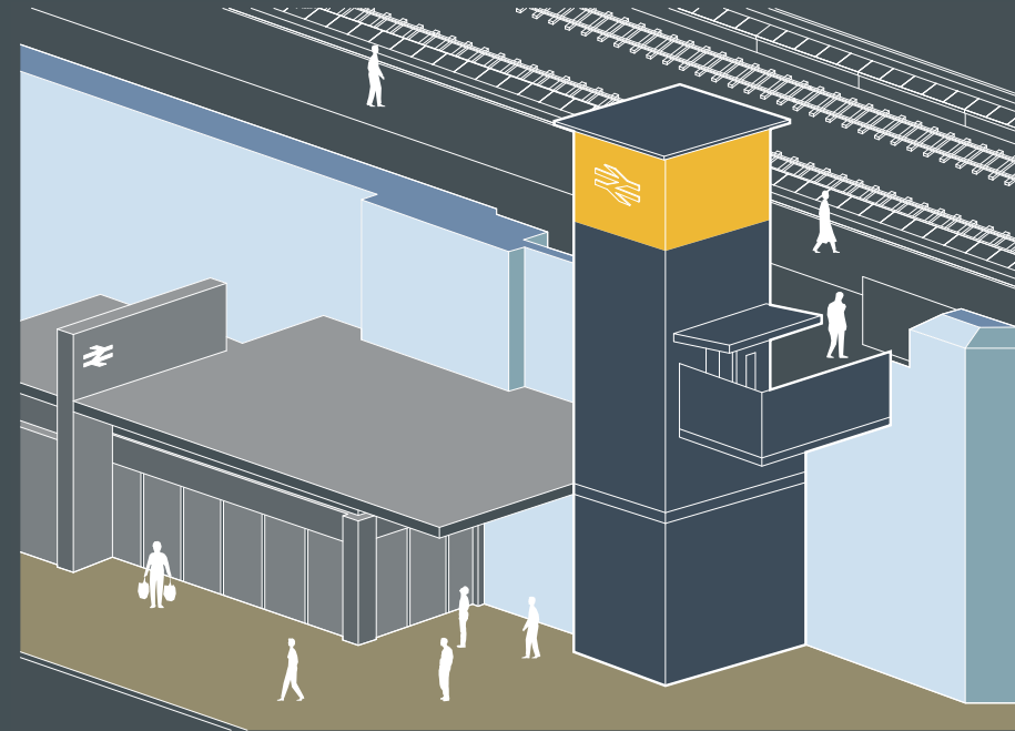
Image B.11 Preferred version - locating the lift machine room elsewhere would reduce space take at street level
