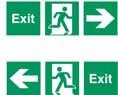
Fig. 46 Examples of an escape route sign, consisting of an emergency exit sign, directional arrow and supplementary text
