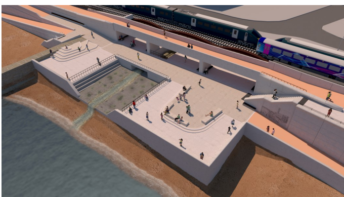
Illustration showing link bridge between sections one and two of the new sea wall, and the stilling basin
