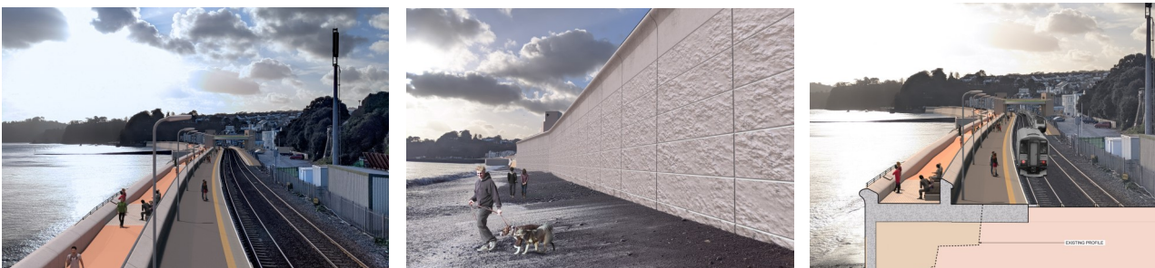
Artist's impression of the new promenade at track level, the new wall from the beach and cross-section of the new and old profiles
