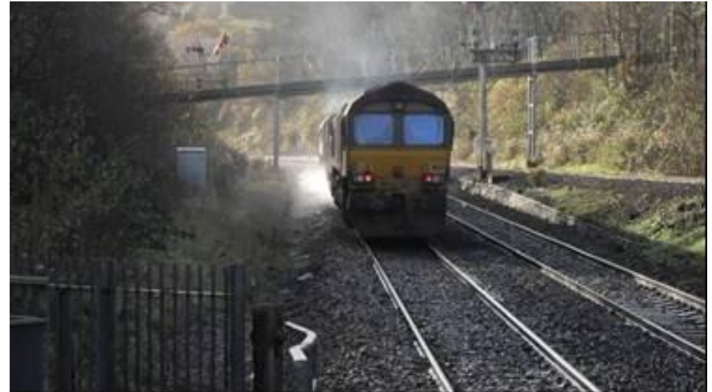
Figure 53 Rail Head Treatment Train in action
