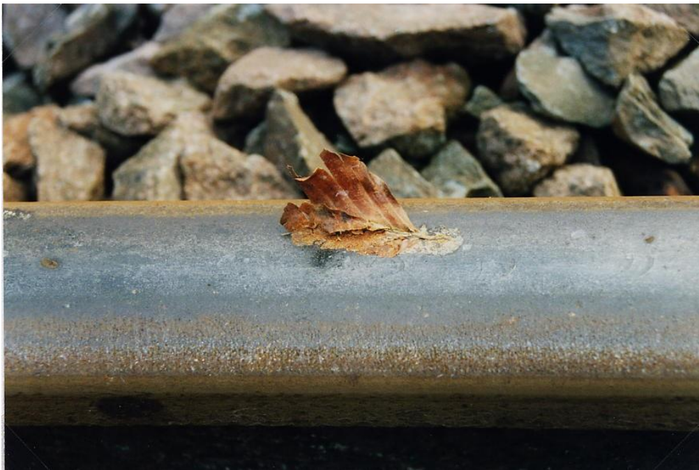
Figure 52 Leaves on the line cause problems with signalling, braking and acceleration
