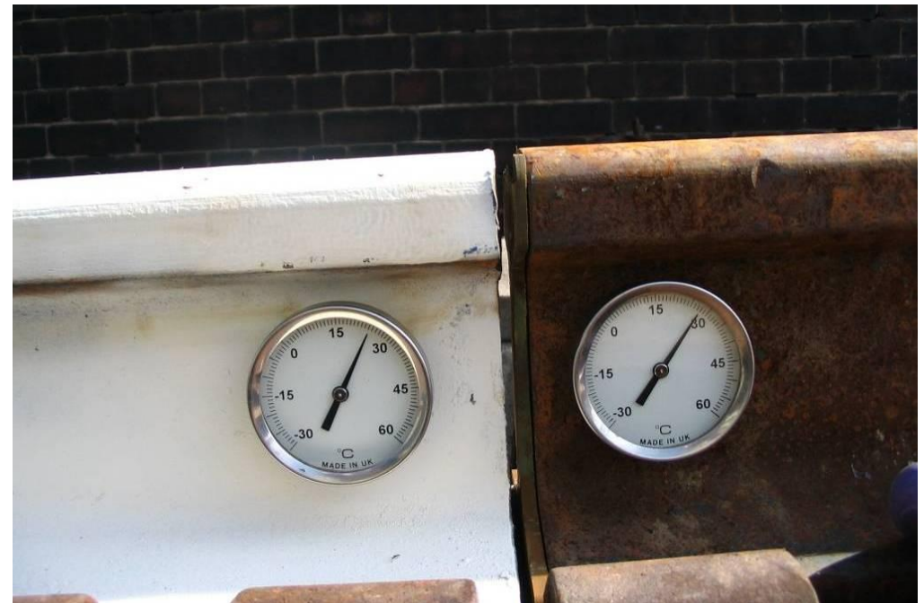
Figure 43 Temperature reduction from painting rails white
