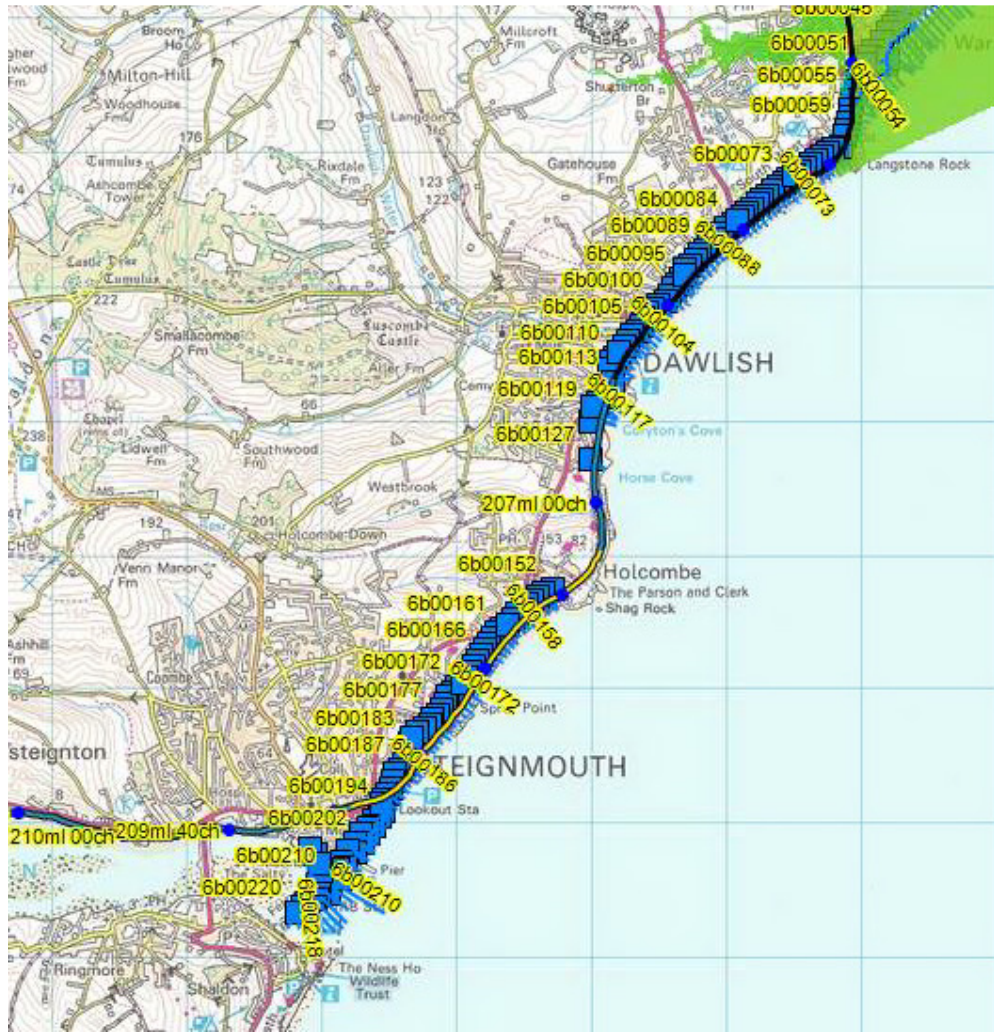
Figure 3-2. Measured beach profile locations from SANDS, the numbers are for beach profile sections
