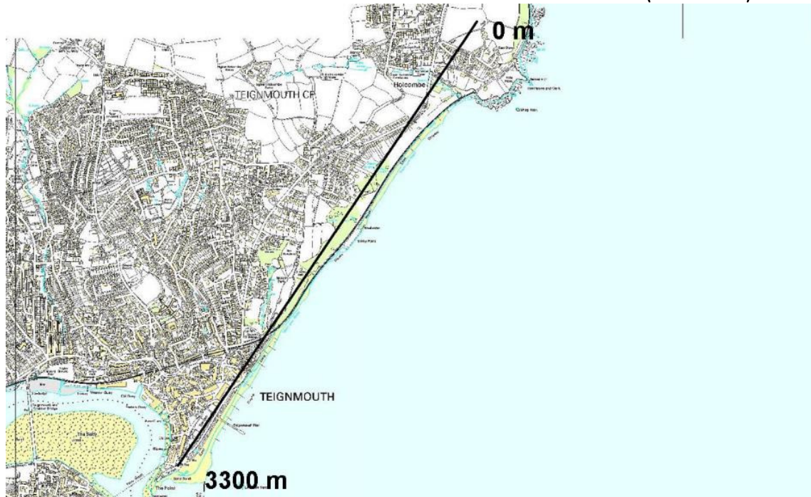
Figure 5-3 Teignmouth LITLINE model set-up. The model extends from Holcombe (northern end) 0 m to the Teign River mouth (southern end) 3300 m.
