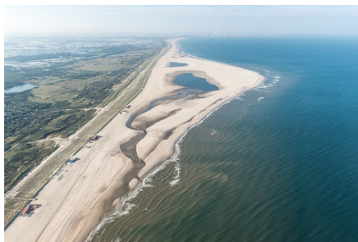
Figure 3-6: Sand engine in development in the Netherlands
