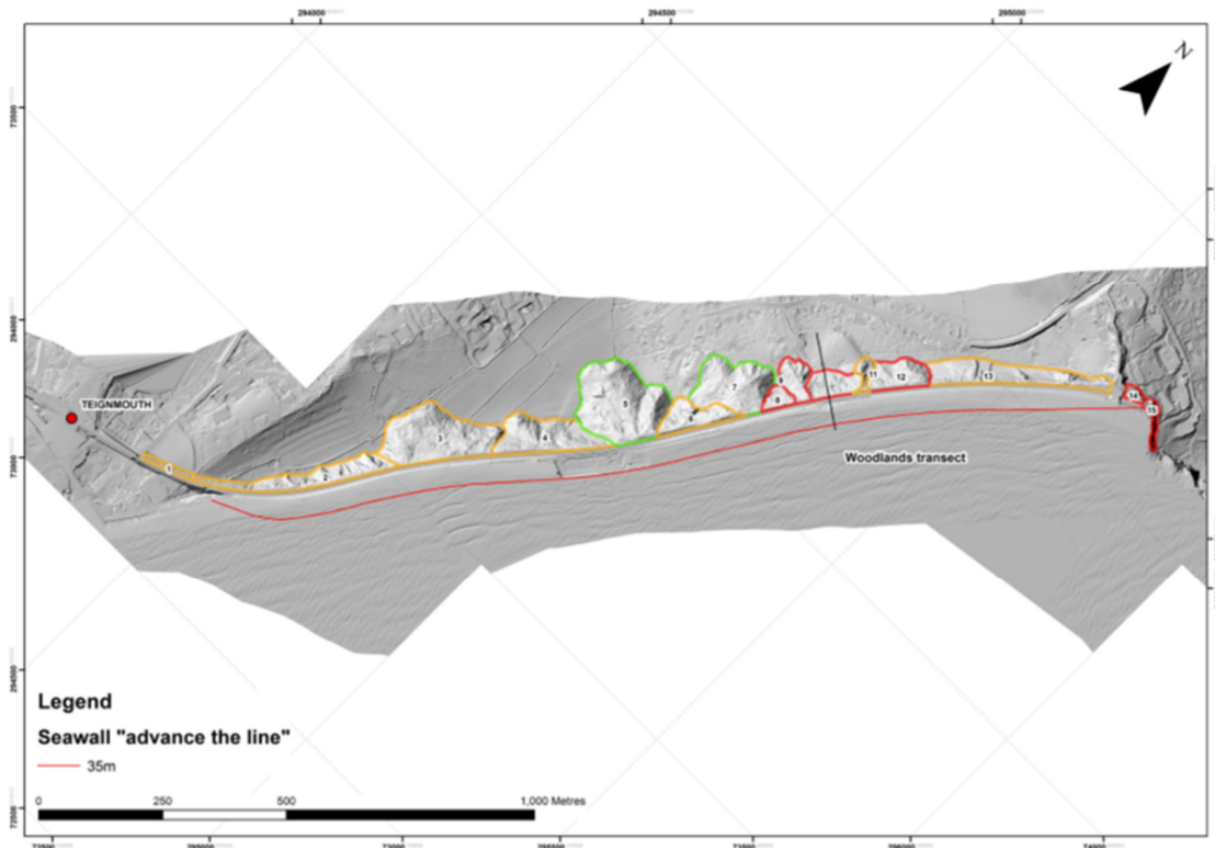
Figure 7-1: Indicative plan showing extents of the 10m and 35m "advance the line" alignments
