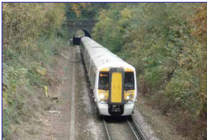
A Class 375 unit heads north towards Tunbridge Wells from Strawberry Hill Tunnel. There are four narrow tunnels between Hastings and Tonbridge where the line was singled to enable standard-width trains to pass through.
