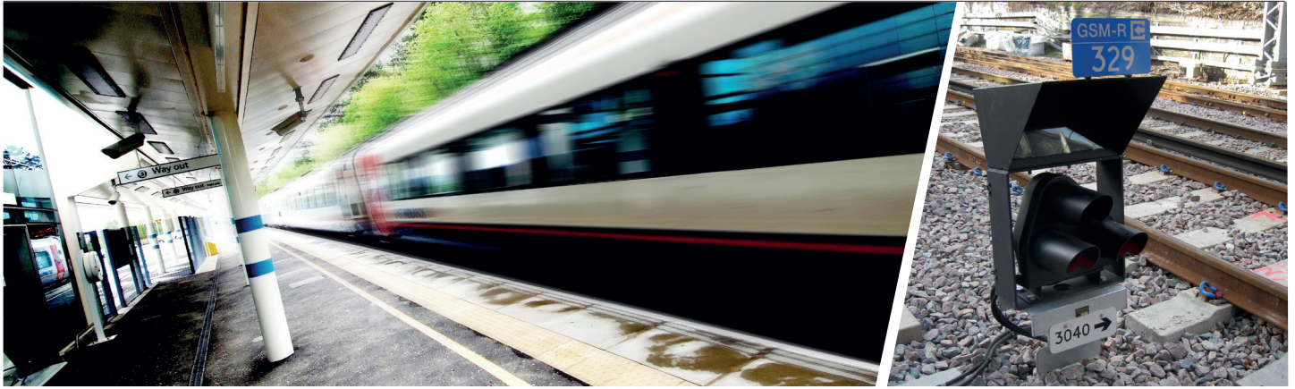
GSM-R sign fitted to Ground Position Light (GPL)
