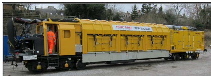
Fig.10 RailVac. The machine has an on board storage for 15 cubic metres of material
