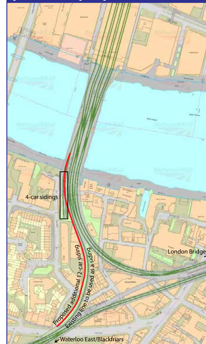
Figure 10.1 - Two carriage siding scheme at Cannon Street
