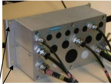
Cab Radio & Gland Box (ARINC Connector) fitment x4 securing points (Torque setting 4Nm)
