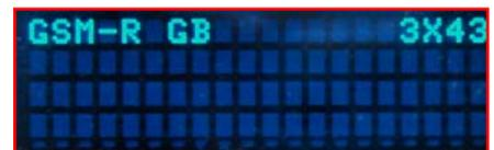
The Emergency Group Call function must be considered live anytime the GSM-R driver's panel (pictured above) is switched on. Normally this will be indicated by the screen having some form of text on it, for example "GSM-R GB", and the buttons will be back lit.
