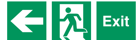
Fig. 46 Examples of an escape route sign, consisting of an emergency exit sign, directional arrow and supplementary text
