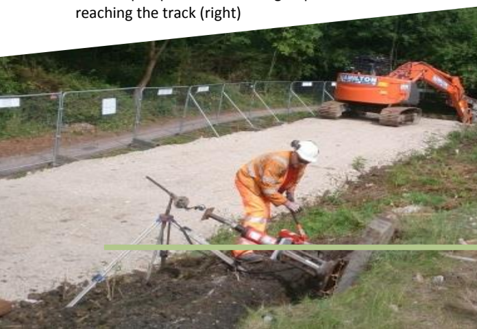
Below: Testing of installed soil nails (left) and a rock slope with draped protection netting to prevent material reaching the track (right)
