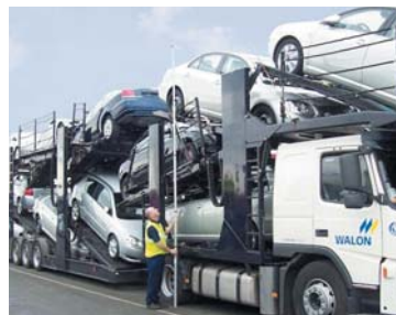
Checking the height of a car transporter using a telescopic measuring device
