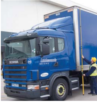
Checking the height of a trailer using a telescopic measuring device
